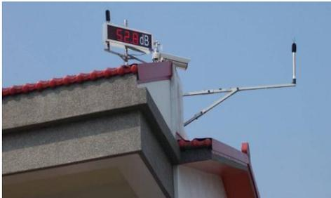
(1) Microphone (2) Weather monitoring Set (3) Camera (4) Central Controller (5) Cables (6) Noise display (7) Support frame
